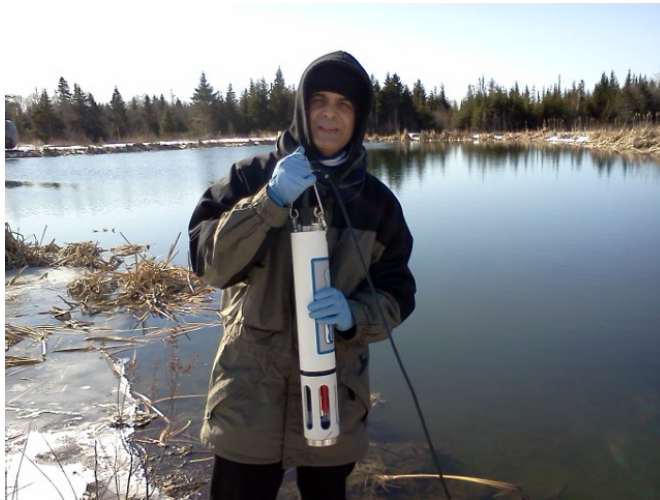
Hamid Khoda Bakhsh and the Hydrolab DS5X Multiprobe to measure water quality (pH, temperature, dissolved oxygen, specific conductivity, etc.) at one of Cooke Aquaculture Inc. hatcheries in New Brunswick, Canada (photo credit: Miko Leavitt).
